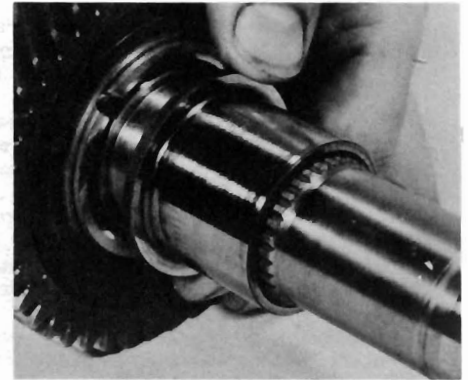
9.13c Fitting the bearing track section to the mainshaft
