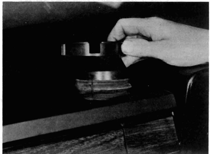
15.3b Removing a fresh air grille seating ring
