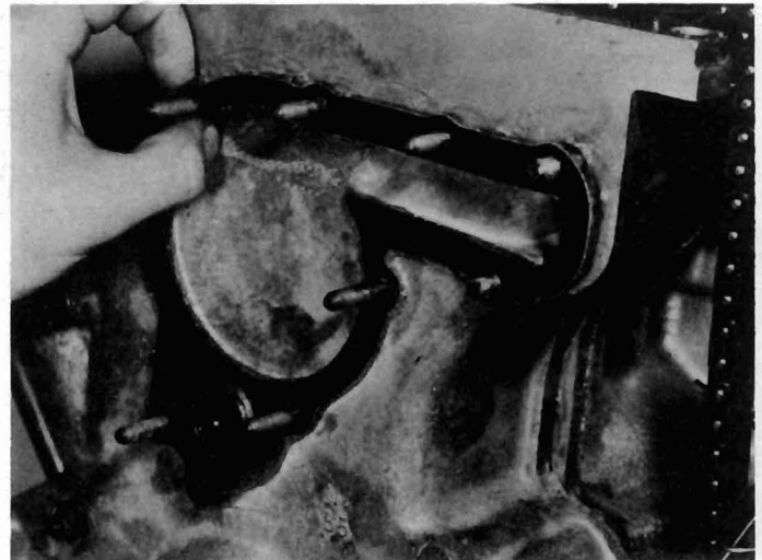
10.7a Locating coolant pump gasket
