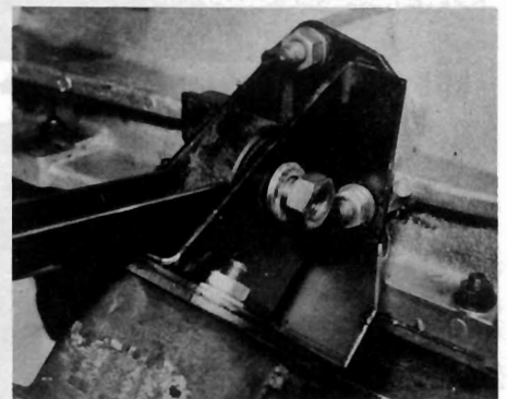
17.44a Fitting carburettor support strut (hot air collector plate not fitted for clarity)
