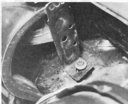
26.4b Wiper motor bracket mounting strut
