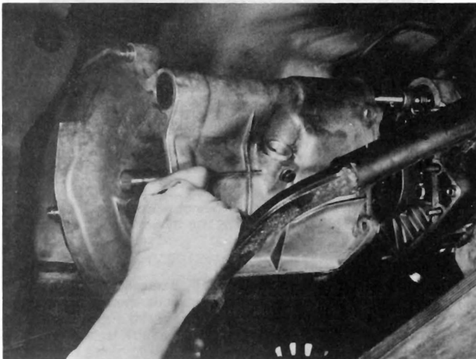
12.5 Installing the gearcase/clutch bellhousing
