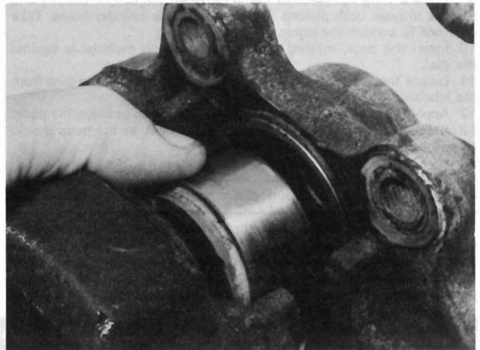
5.6 Removing a caliper piston
