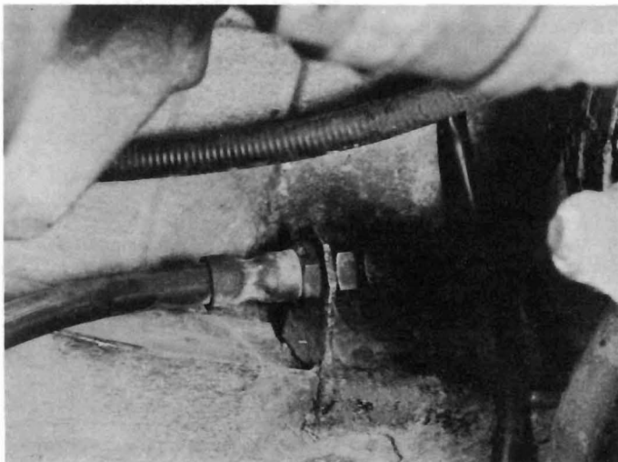
11.7 Typical brake hose/pipe connection
