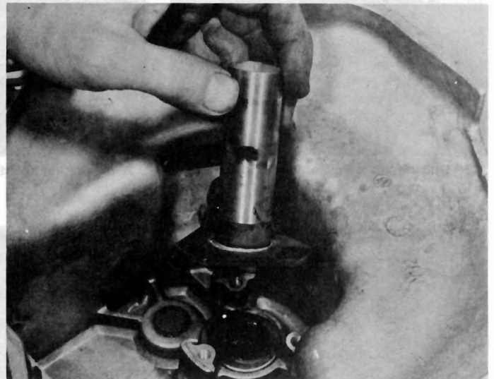
9.35b Fitting release bearing guide sleeve
