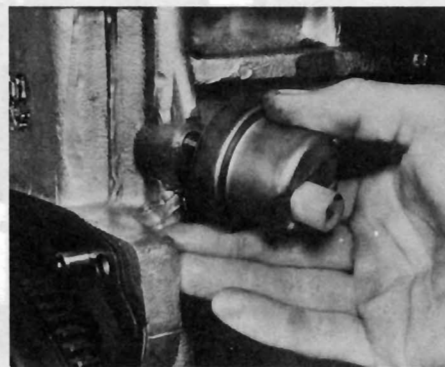
17.34a Fitting the oil pressure sender
