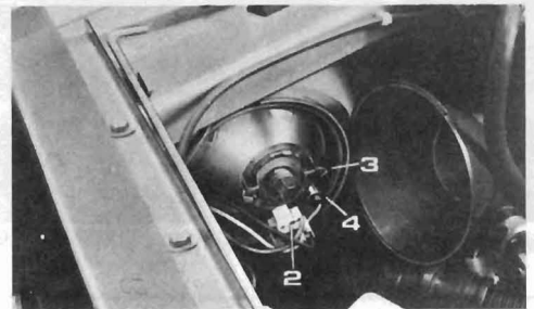
Fig. 9.10 Headlamp protective cover removed (Sec 16)
