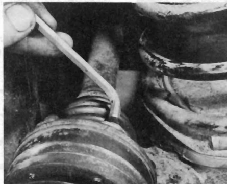
5.2a Unscrewing driveshaft outboard end flange screw
