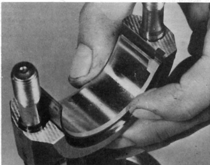
9.15 Fitting a connecting rod bearing shell
