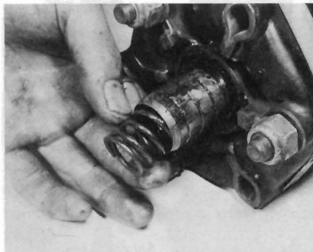
3.7b Removing coupling bush coil spring
