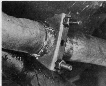
11.22a Exhaust section clamp
