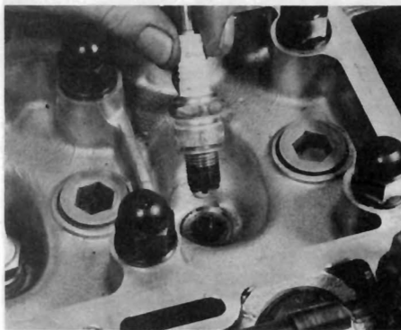
17.30 Fitting a spark plug
