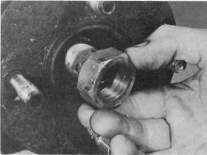
5.14 Fitting rear hub nut
