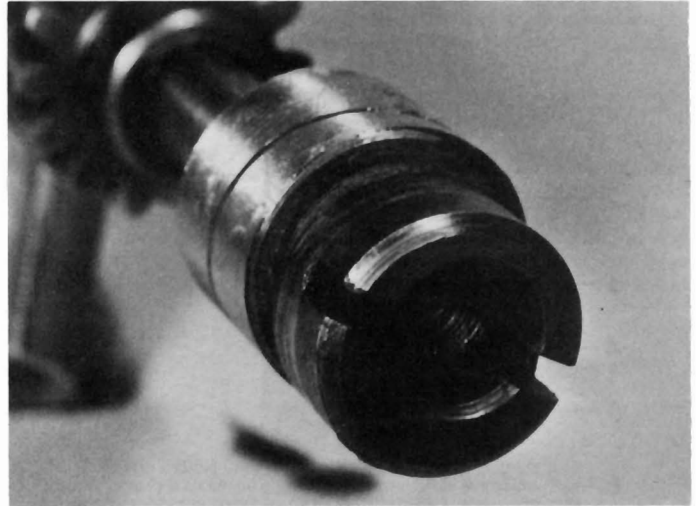
6.6 Distributor driveshaft offset dogs
