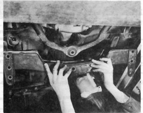
13.13a Raising the transmission front crossmember into position
