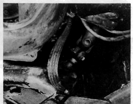
18.5 Earth strap (flywheel housing to body)
