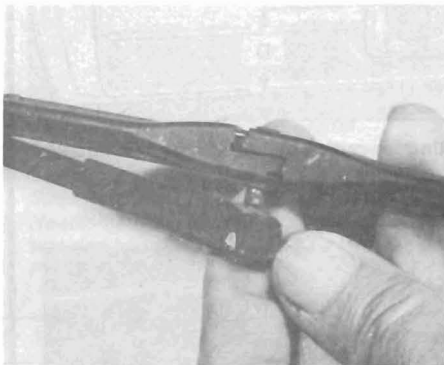
25.2 Separating wiper blade from arm
