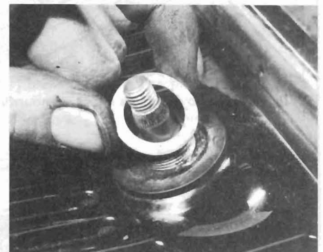
26.3b Wiper spindle gasket and washer
