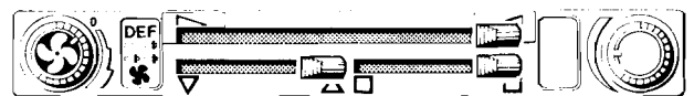
Warm air flow to outlets B (screen demisting) as well as to outlets C
