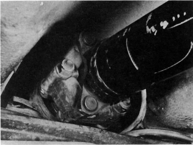
2.10 Propeller shaft front coupling
