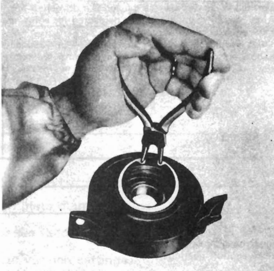
Fig. 5.13 Extracting the centre bearing circlip (Sec 3)
