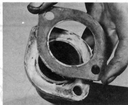
16.9b Exhaust downpipe flange gasket
