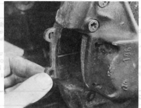
3.6 Withdrawing the disc pads
