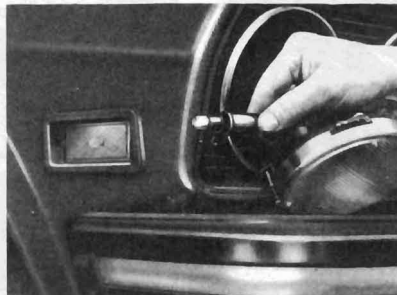
Fig. 9.18 Front side marker lamp bulb and holder (N America) (Sec 19)
