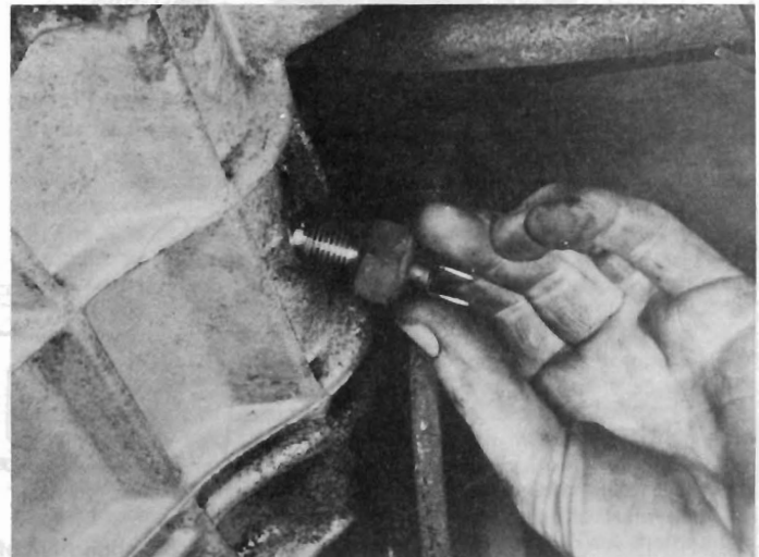
12.8 Screwing in the reversing lamp switch
