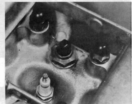
17.34b Oil temperature switch
