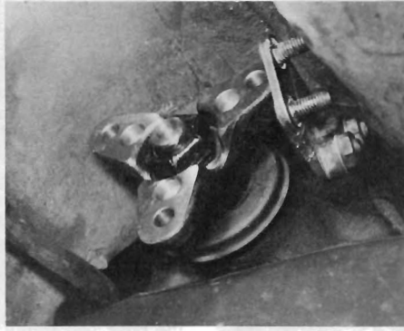
3.20a Modified type of clutch yoke
