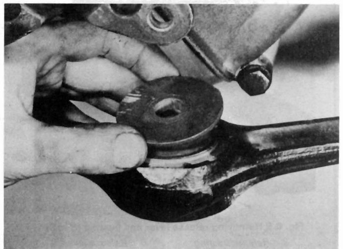
6.4 Transmission crossmember mounting. Note spacer
