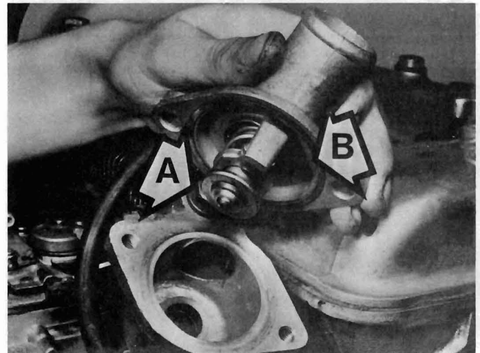
5.2 Removing thermostat housing cover. Note thermostat housing bleed screw (A) and O-ring seal (B)
