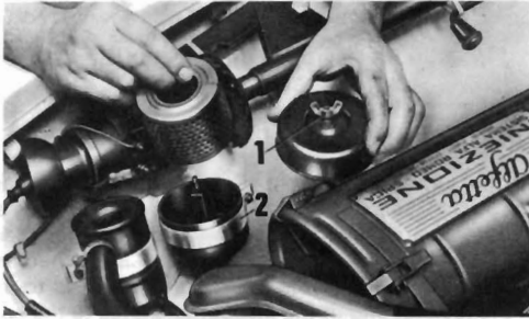
Fig. 3.23 Air pump air cleaner (Sec 33)
