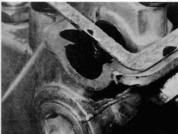
3.18a Camshaft cover gasket and sealing plug
