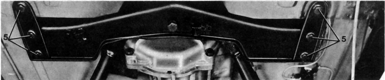
Fig. 7.4 Rear axle crossmember bolts (5) (Sec 5)
