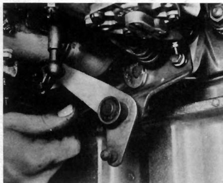
16.3d Accelerator control rod, bellcrank and bracket under inlet manifold
