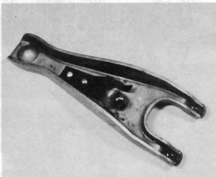
3.10 Reverse side of clutch release lever
