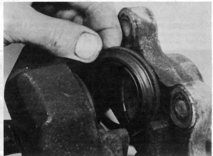
5.12 Fitting a caliper dust excluder
