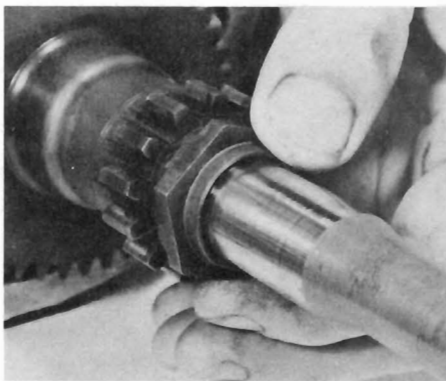
9.5 Screwing on the input shaft nut
