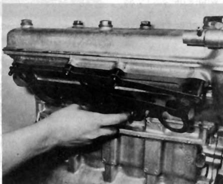
16.3b Inlet manifold gasket
