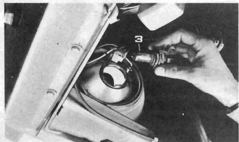
Fig. 9.11 Headlamp bulb and holder (3) removed (Sec 16)
