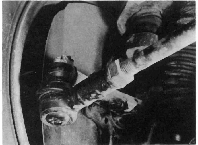
14.2 Track rod end balljoint
