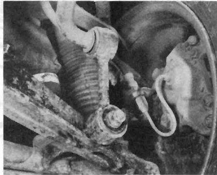
6.1 Anti-roll bar end link
