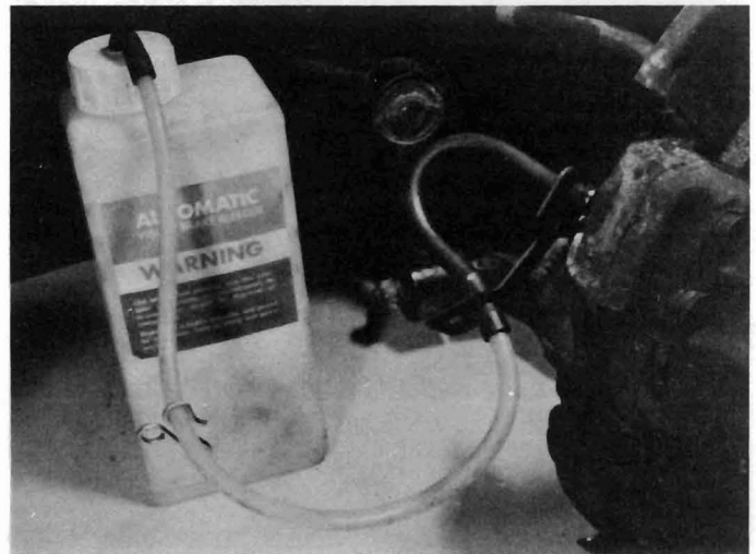
12.12 Bleeding a caliper with a one-way valve kit
