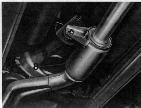
Fig. 1.18 Exhaust front section flexible mounting (Sec 11)
