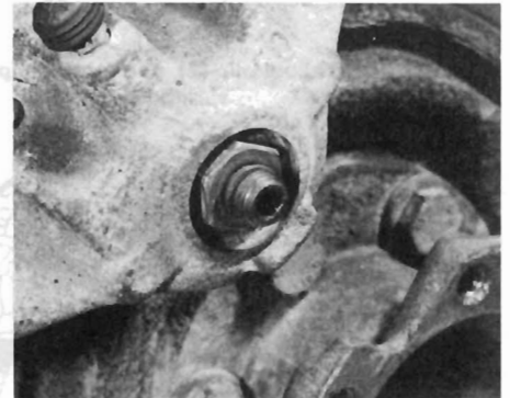
4.4 Rear disc pad adjuster screw showing Allen key hole
