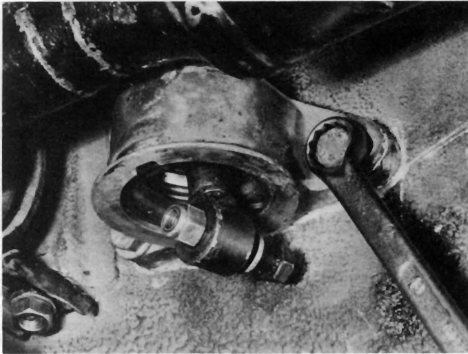
2.13 Gearchange lever ball socket housing
