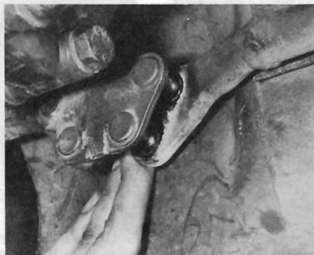
2.7 Gearchange link rod attachment to gearbox selector lever
