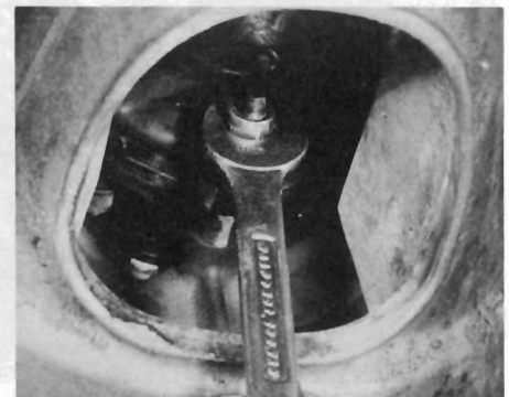
2.9 Unscrewing a propeller shaft front coupling nut
