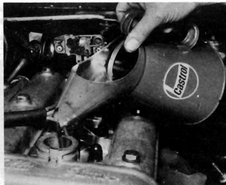
Topping up the engine oil
