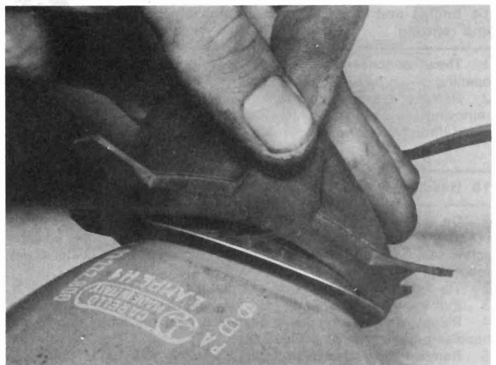
16.1 Removing headlamp rear cover
