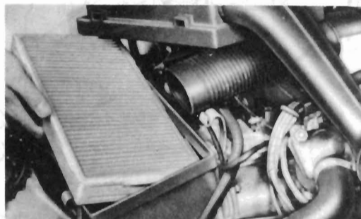
Fig. 13.4 Air cleaner on later carburettor models (Sec 5)
