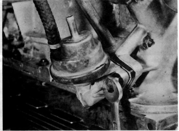
17.36b Bolting on the fuel pump
