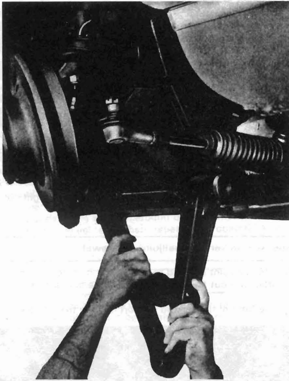
Fig. 10.7 Removing the suspension lower arm (Sec 8)
