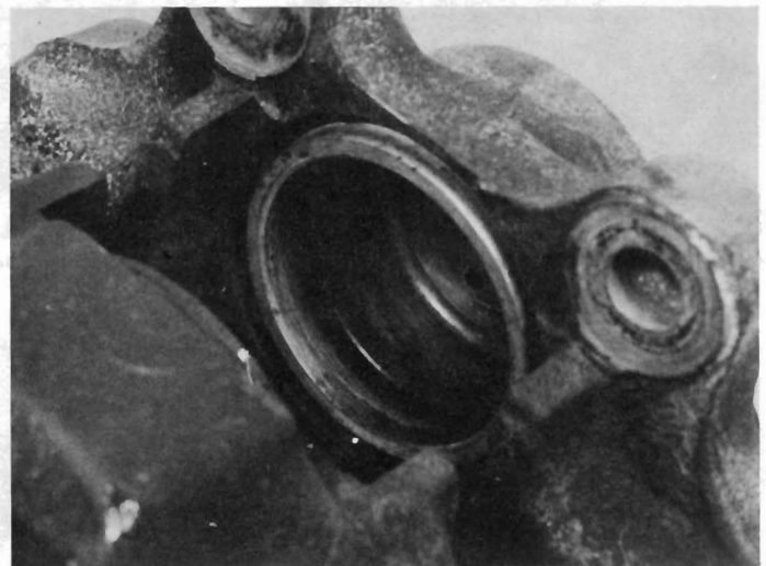
5.9 Piston seal in caliper cylinder bore
