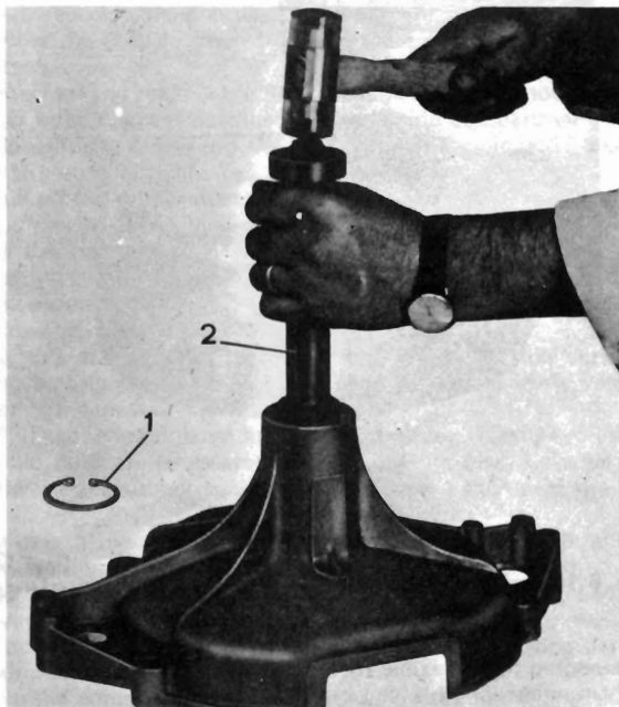
Fig. 6.8 Direction of removal of front bearing (Sec 3)
