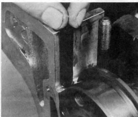
17.11d Crankshaft rear bearing sealing strips
