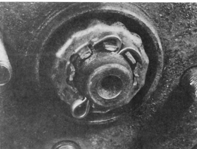
5.15b Rear hub split pin correctly fitted
