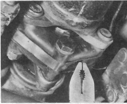
3.13 Removing propeller shaft coupling band
