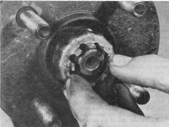
5.15a Fitting rear hub nut lock
