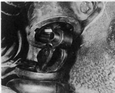
2.6 Gear lever disconnected from gearchange link rod
