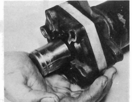
3.11b Using a socket to install coupling to shaft
