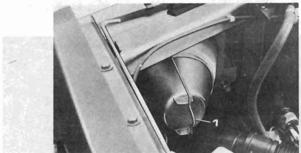
Fig. 9.9 Headlamp protective cover and clip (1) (Sec 16)
